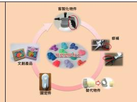
The shape-memory technology is to make the plastic polymer material to form the shape that you want, for create your own idea. A special ingredient is added to the plastic, which makes the plastic shape-memorable. It looks simple but it can be different shape according to the temperature changes. PIDC has developed a series of shape-memory materials for plastic clay product, which can be easily used for DIY home repair.
